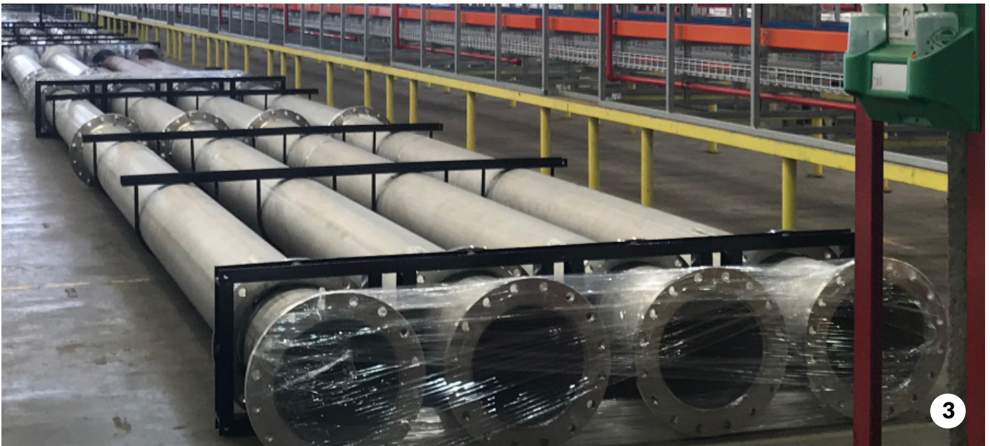
Figure 20: Modules pre-assembled in the factory
