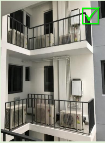
Fig. 4-36 Safety barrier is provided for the AC ledge
