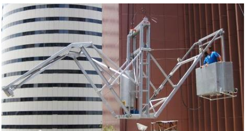
Fig. 3-6 A pantograph cradle can enable access to facades beneath projections or in recesses
