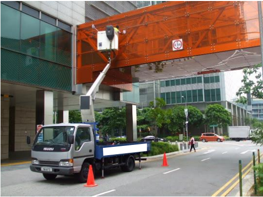
Fig. 3-21 An example of a truck-mounted boom lift
